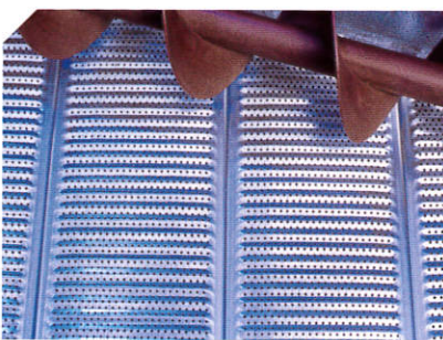
Built-in corrugation on planks increases strength and rigidity. Round perforation (0.93") design is smooth and easy to sweep.
